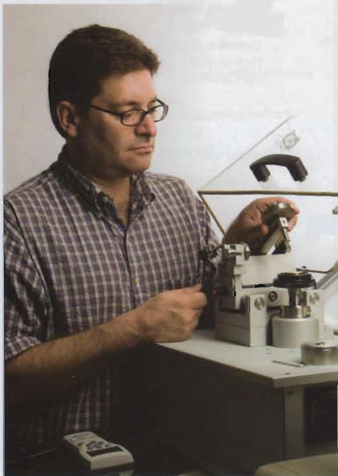
Dr. Jeffrey Lince prepares to make pin-on-disk friction and wear measurements. This testing is performed to measure the sliding coefficient of friction between two materials under ambient or purged atmospheres. (Courtesy of The Aerospace Corp.)
